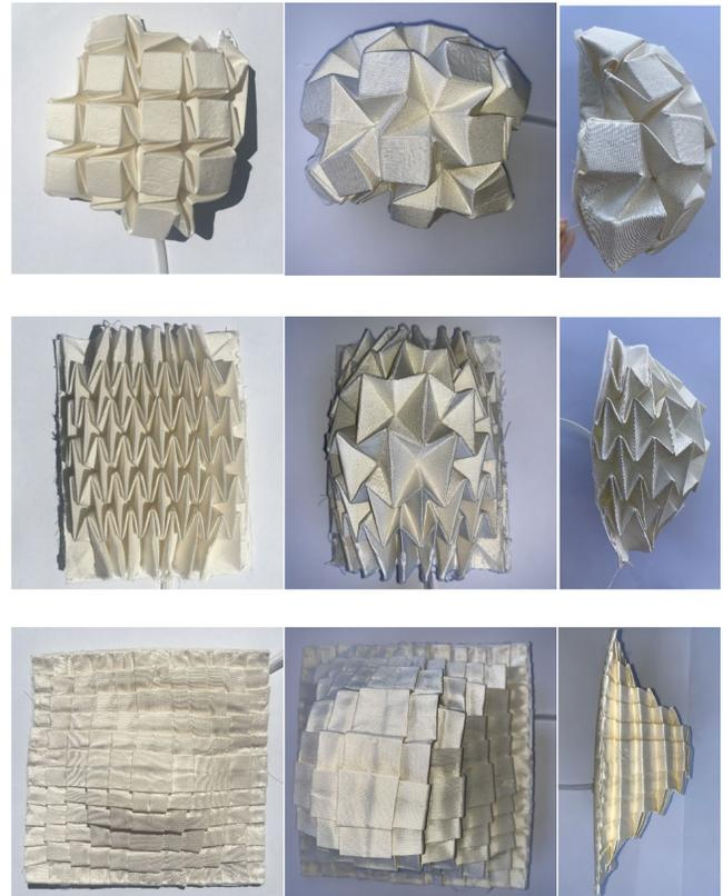
**Figure 1: Eight-Crease Waterbomb (Top row); Six-Crease Waterbomb (Middle row); Pyramid (bottom row); non-inflated, view from the top (left column), inflated view from the top (middle column) and the side (right column).**
