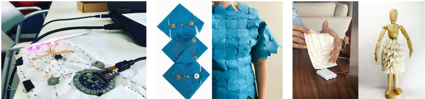
Figure 1: Example toolkits for wearables. (Left) An e-textile prototype built with Arduino Lilypad[2]; (middle) Wearable bits, a toolkit for wearable e-textiles [16]; (right) shape changing fabric samples for exploring interactive fashion design [31].
