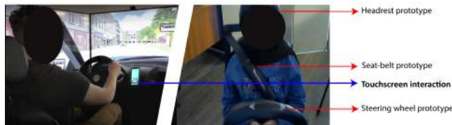
Figure 5: Final implemented prototypes (right) versus the touchscreen interaction through the smartphone (left) when each is situated on the driving vehicle simulator.
