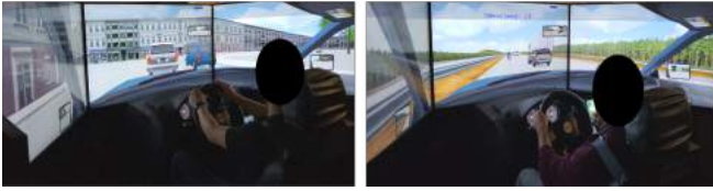
Figure 8: The two scenarios, i.e. city and expressway, were used for the e-textiles and screen-based interactions during the study. The left figure shows the city scenario where the participant is interacting with the steering wheel sensor, while the right figure shows the expressway scenario where the participant is interacting with the multitouch screen.
