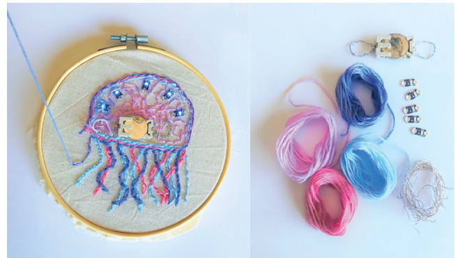
Figure 7: An e-textile jellyfish sketch made with the punch needle and being pulled out by one thread (left), the threads wrapped up for reuse after pulling them out (right).
