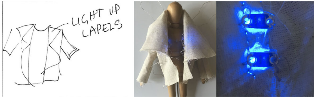
Figure 9: With practice practitioners can use the punch needle to quickly prototype 3D objects in-situ without a tension frame. In this example, a wearable jacket concept goes from sketch (left), to quick mock-up using the punch needle (middle), with a close up of the punched stitches (right)
