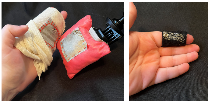
Figure 5: Left: First iteration of the touch switch which replaces the cardboard with a pillow. Right: Small version of the touch switch with conductive thread replacing the conductive fabric.
