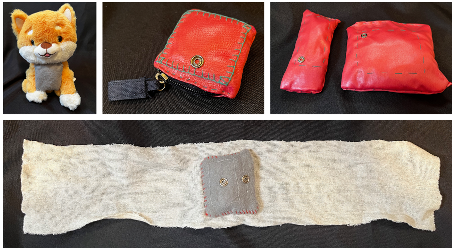
Figure 7: Four different iterated push switches. Top Left: The first switch has the push switch sewn into the chest of the dog toy. Top Middle: The second switch has a zipper sewn into the switch. Top Right: The third includes two different sizes of push switches. Bottom: The fourth switch has a pillow switch attached to a stockinette.
